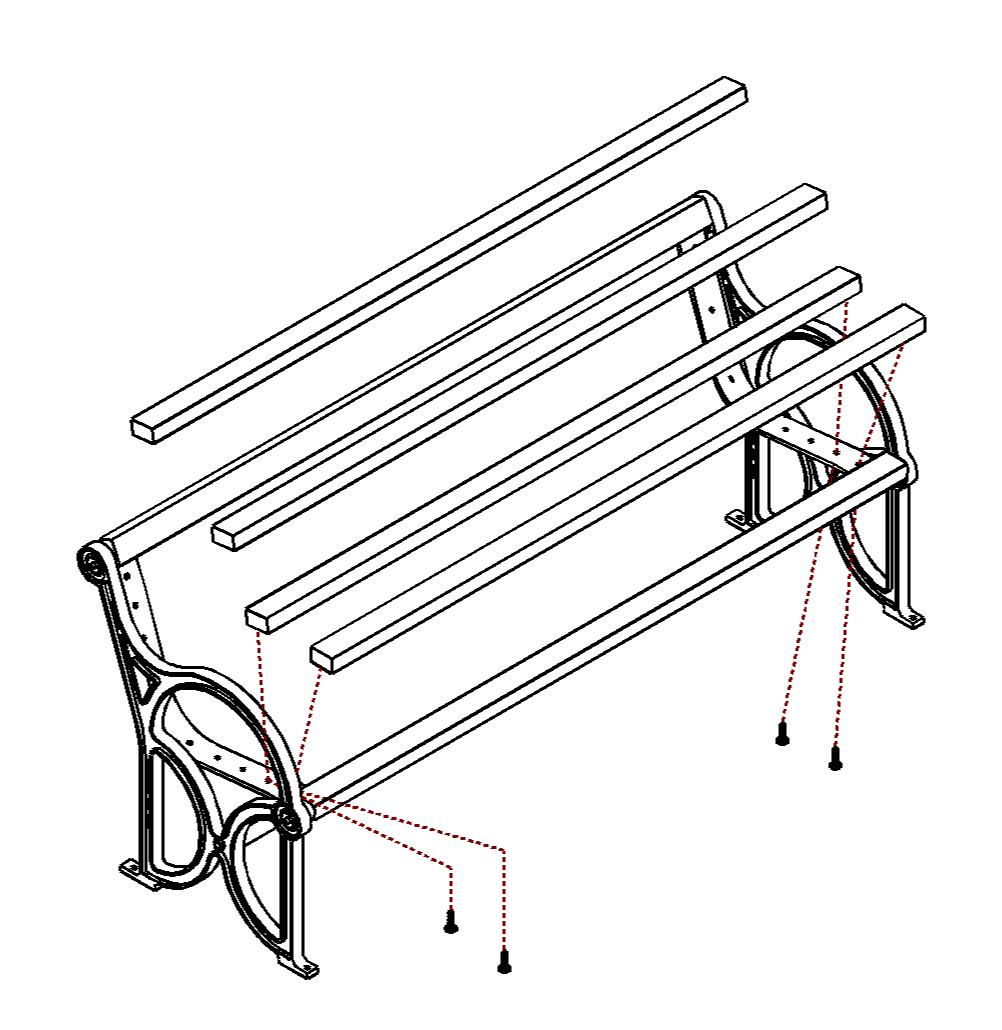
For step 4 and 5 use lag screw combination (parts A & B) as shown:
