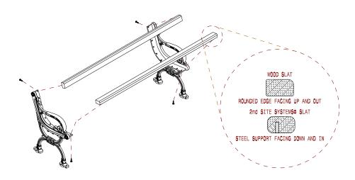
For steps# 2, 4 & 5 use lag screw combination (parts A & B) as shown:
