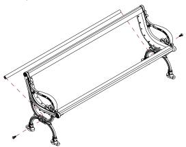
For step# 3 use hex bolt combination (parts D & E) as shown:
